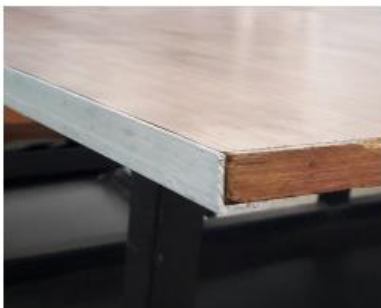
Steel L section fixed on the parallel sides of board
